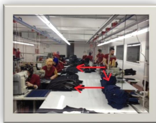
Image 4. Distance that a Trousers Pocket is Prepared and Sent for Sewing before the Adjustment
