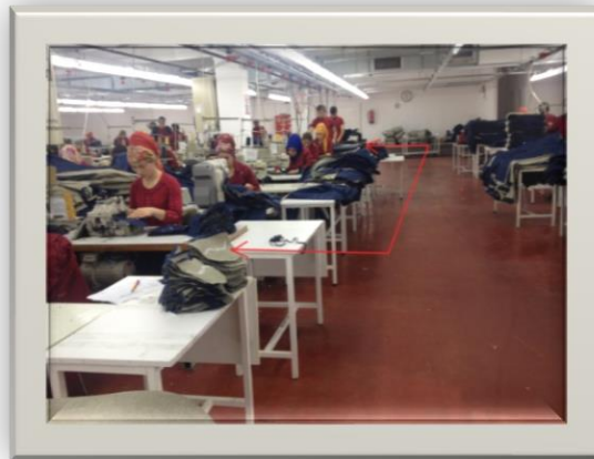
Image 3. Distance that the Trousers Pocket is Prepared and Sent for Sewing before the Adjustment
